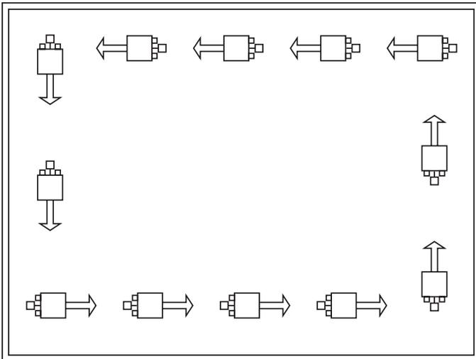
UNIT HEATERS are suspended overhead and in warehouse, are very often located around the perimeter as shown. Mounting heights are variable with unit size. Downturn nozzles are available to increase standard mounting height. Unit heaters may be used to circulate air in the summer months.
