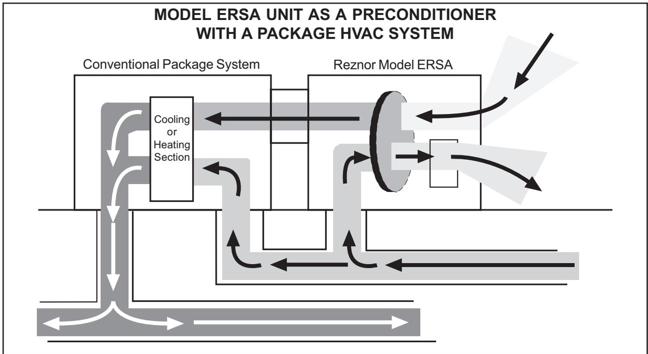
the winter months as in summer with the added benefit of adding moisture to the outdoor air. This reduces the amount of moisture that will need to be added to maintain the minimum indoor relative humidity levels.
