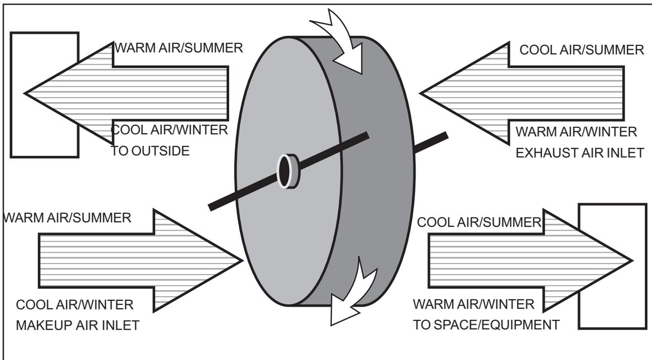
into the incoming fresh air stream. The desiccant will “absorb” molecules depending on
