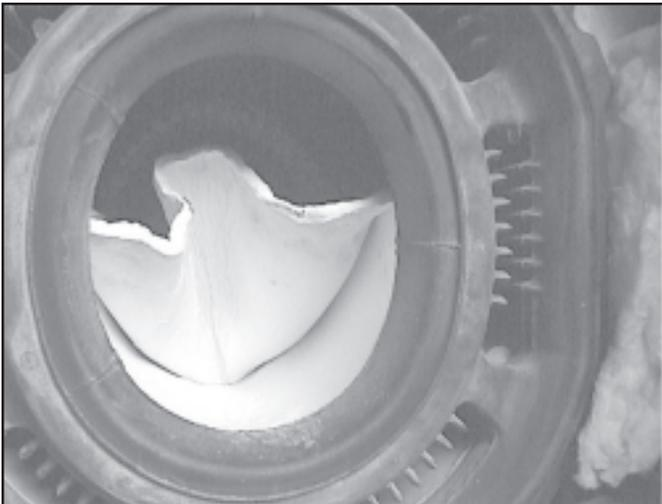
**Figure 5 - Position the liner sleeve so that the front edge is as close as possible to the front edge of the chamber. Working from the bottom up, mold the liner to the combustion chamber.**
