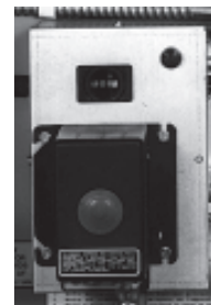
Phelon Controller with one light and hour meter
