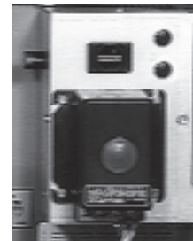
Phelon Controller with two lights and hour meter
