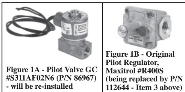
Disconnect the 1/4" pilot tubing from both the pilot valve and the pilot regulator. On the pilot regulator, remove the 3/8" x 1/8" NPT hex bushing from the inlet side. Save this bushing as it will be used when installing the new pilot regulator.
