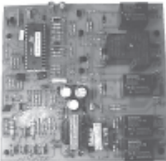
Figure 1 - Hot Surface Ignition Module, P/N 157953, in all Replacement Kits
