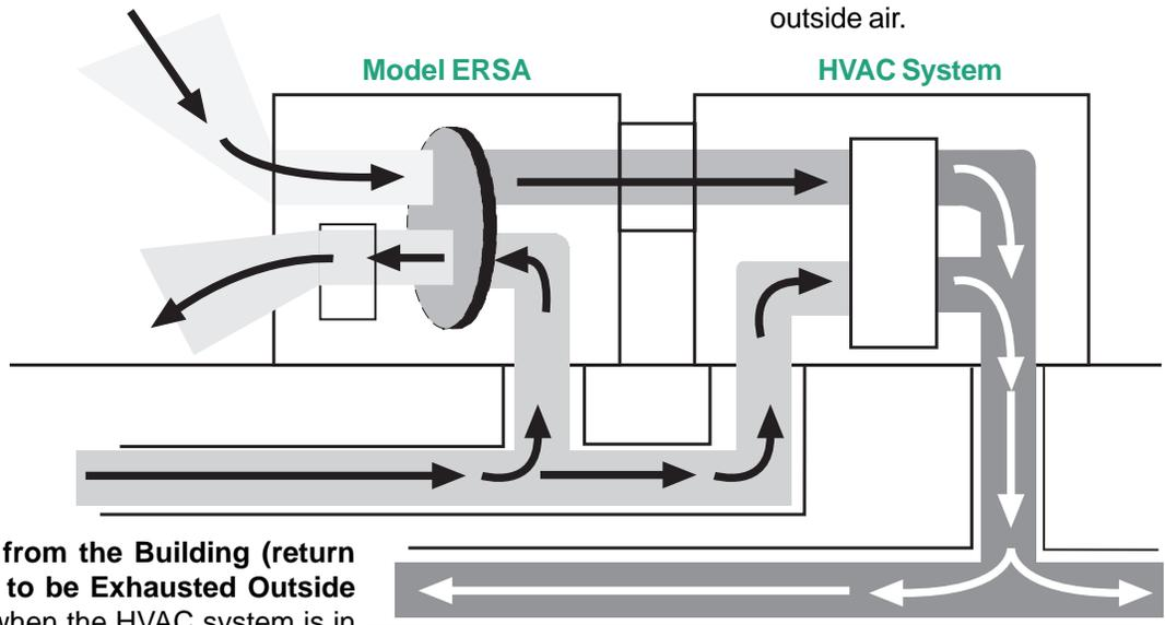
**Air from the Building (return air) to be Exhausted Outside** — when the HVAC system is in the heating mode, the energy recovery wheel “recovers” the heat and humidity in the return air by transferring it to the incoming air; when in the cooling mode, the wheel transfers the unwanted heat and humidity from the incoming air to the airstream being exhausted to the outdoors.
