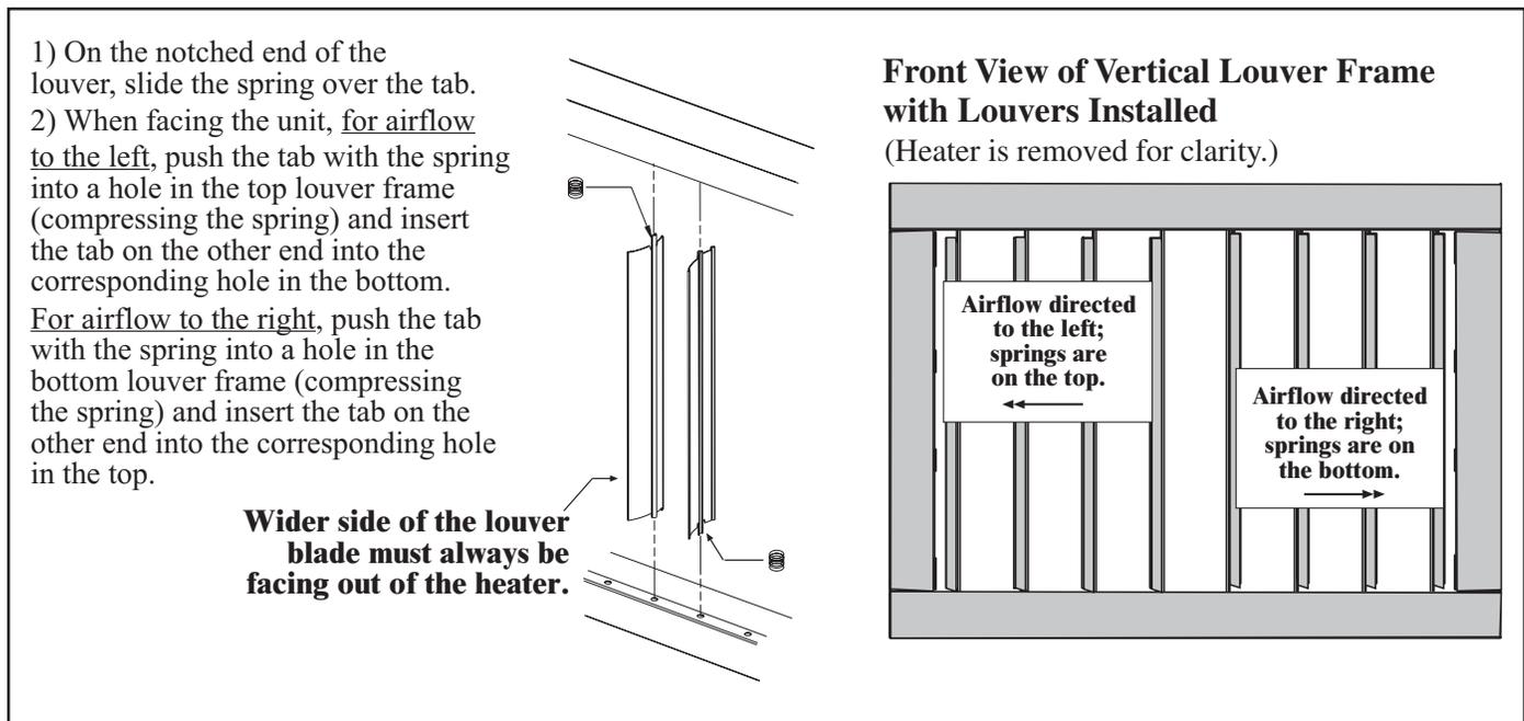
5. Adjust the horizontal and vertical louvers to provide the desired throw pattern.
