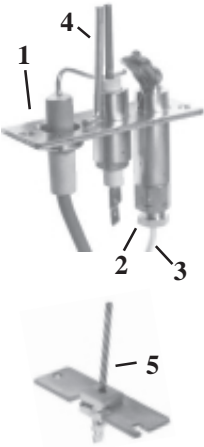
Figure 9 - Vertical Spark Pilot for Models RPV, RPBE, RPVE, RPVJ, RPVAK, HRPV, HRPBE, HRPVE, CRPV, HCRPV, CRPBE, HCRPBE, CRPVE, HCRPVE; CRPVAK prior to Series 6 and RCG 7-12/, 10 ton equipped with G60 or G67 ignition Controller
