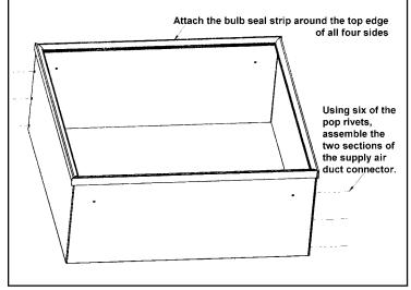
STEP 5 - Using four sheet metal screws, attach one of the blower supports (removed from the blower in STEP 2) to each side of the supply air duct connector assembled in STEP 4.
