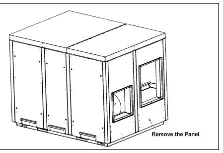
STEP 2 - Remove the cover and plug, revealing the opening in the cabinet bottom panel.
