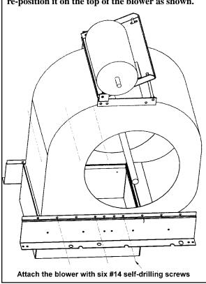
STEP 7 - Position the sub-assembly (duct connector, two blower supports, and blower) as illustrated with the duct connector in the opening in the cabinet bottom panel.
