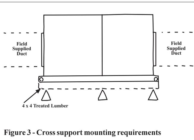
**Figure 3 - Cross support mounting requirements**
