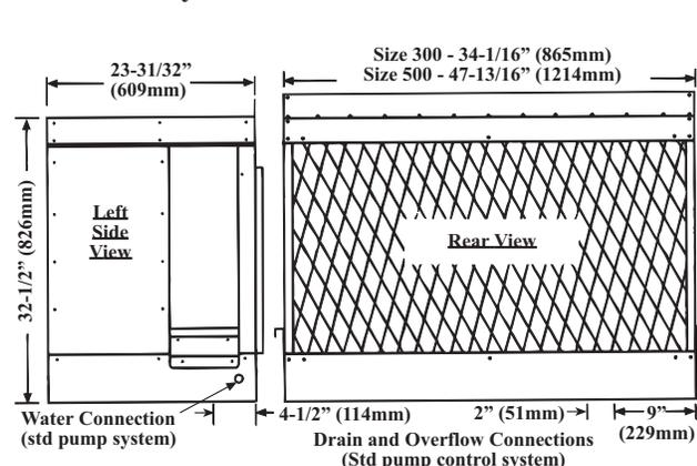
**Figure 18 - Factory-installed Evaporative Cooling Module Option on Models ADF/ADFH 300 and 500**
