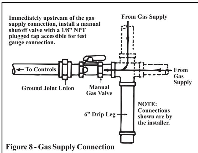
**Figure 8 - Gas Supply Connection**
