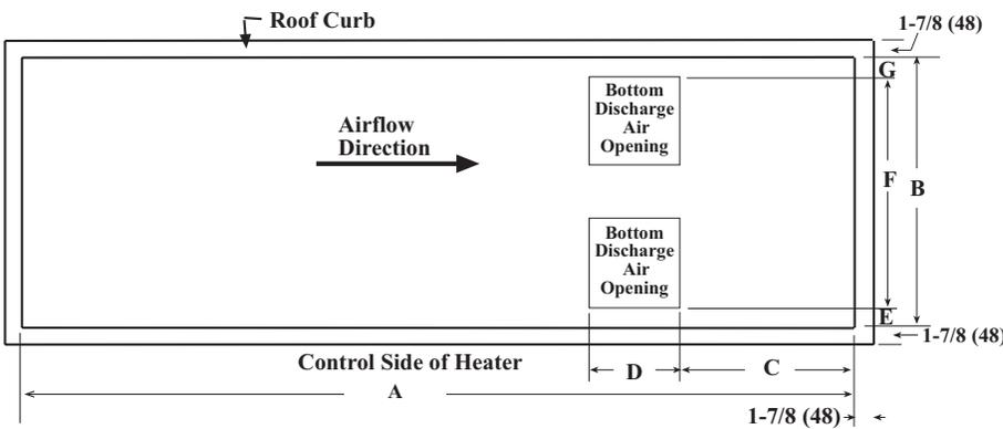
**Figure 5 - Vertical Duct Connection in Relationship to Reznor® Roof Curb**
