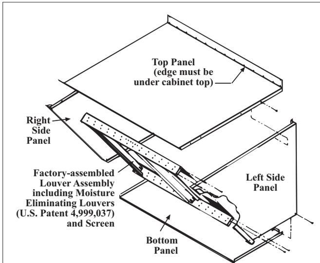
**Figure 12A - Assembly Drawing of Option AS2, Outside Air Hood Without Filters**
