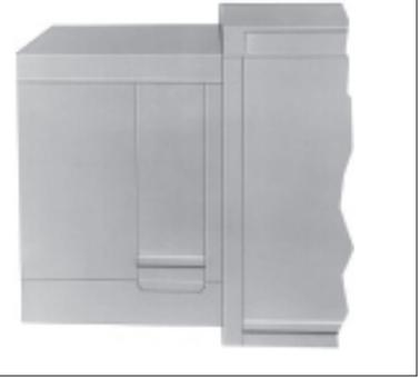
**Models ADF/ADFH 700/1200** - The evaporative cooling module for Sizes 700 and 1200 is assembled at the factory and shipped separately for field-connection to the makeup air system cabinet. The shipped separate option includes the cooling module, an adjustable base, and the transition ductwork between the cooling module and the cabinet. Complete installation instructions including dimensions are packaged with the evaporative cooling module package.
