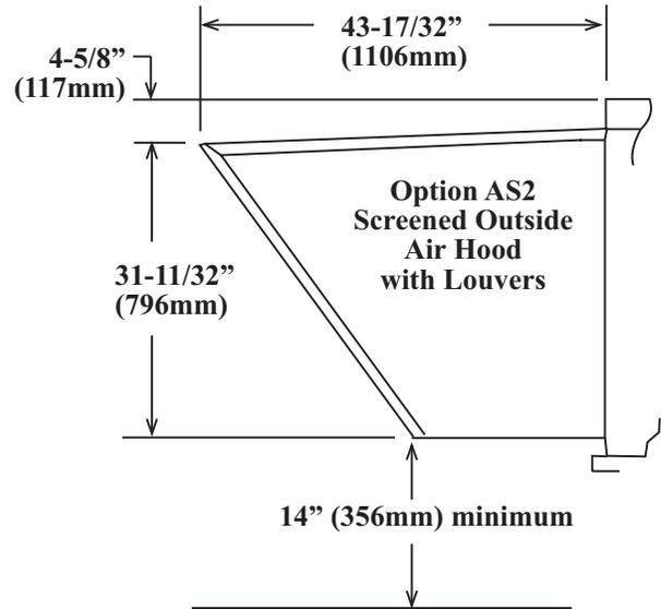
**Figure 1B - Optional Horizontal Discharge Damper - applies to all Sizes**
