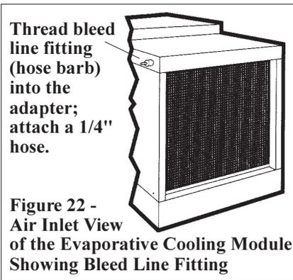
Discharging a quantity of water by "bleed off" will limit the concentration of undesirable minerals in the water being circulated through the cooling module. Minerals buildup because evaporation only releases "pure water vapor" causing the concentration of contaminants in the water to increase as the evaporation process continues to occur.
