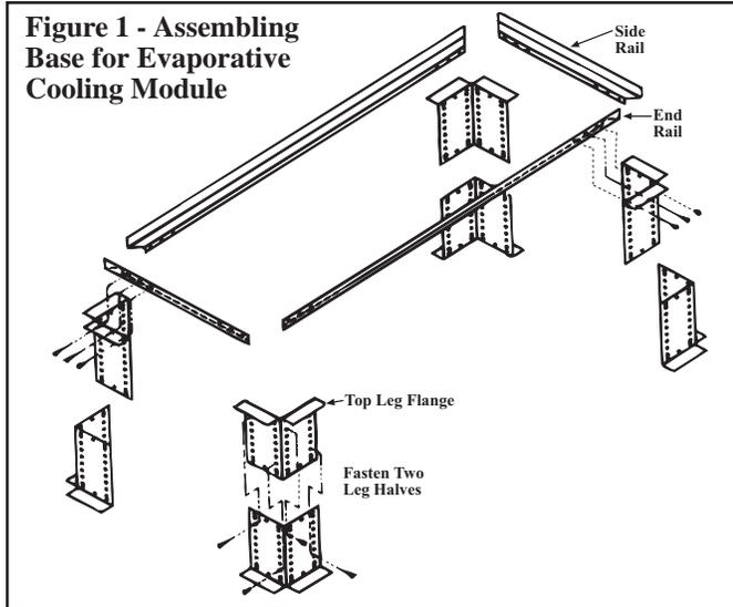
Position the four assembled legs in a rectangular pattern corresponding to the size of the cooling module (see dimensions, page 1). Consider minimum length of transition duct (page 2) when positioning the cooling module base. Depending on the type of roof, it may be necessary to set the legs on a weather-resistant, solid wood or metal base.
