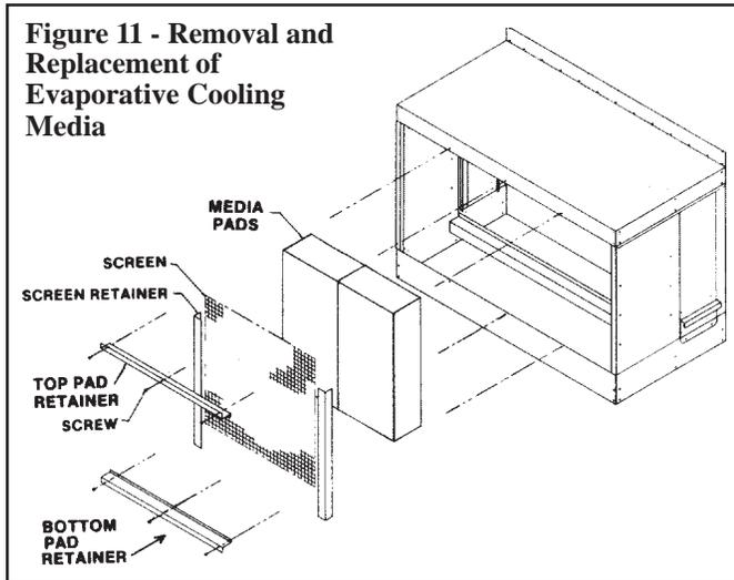
**IMPORTANT: Cooling media is made up of two different sheets of cooling material. Each has its own unique angle. When replacing the cooling media, BE CERTAIN the 45° angle slopes downward toward the incoming outside air. If the media is not installed properly, water blowoff from the media pads will occur.**
