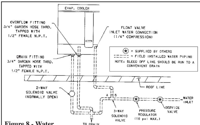
**Figure 8 - Water Connections including Optional Drain and Fill Kit**
