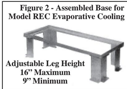
Place rail sides on the **inside** of the top flange of the leg assemblies. Using the bolts and nuts provided, bolt the side rail to the top three holes located on the legs just below the top flange. Repeat on the remaining three legs. Tighten nuts securely.
