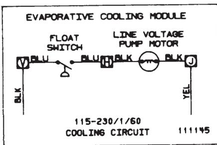
**Diagram of Evaporative Cooling Module Factory-Installed Wiring -- 208/1-3/60**
