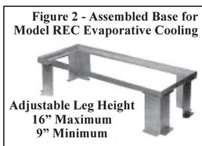
type of roof, it may be necessary to set the legs on a weather-resistant, solid wood or metal base. Module must be level. Place rail sides on the **inside** of the top flange of the leg assemblies. Using the bolts and nuts provided, bolt the side rail to the top three holes located on the legs just below the top flange. Repeat on the remaining three legs. Tighten nuts securely.
